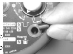
For all Group Cameras *other than* **R-TTL** , **R-S** , **R-M** leave the Advanced Cancel Circuit **ON**, by *not* installing the magnet.
