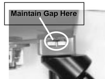
There is a 6mm threaded socket in the base of the strobe. Whichever attachment system you use always be sure the bolt length is not too long. If the bolt is too long and is screwed down so that it contacts the housing body, the strobe may be damaged. When screwing in, always make sure there is a gap between the end of the bolt and the strobe body.
