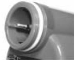
When the battery box cap is fully screwed down and seated on the O-ring surface, look at the O-ring through the transparent edge of the cap. You should see a continuous, uniform contact line (the “witness line”) between the cap and O-ring. If the contact line is not uniform, or twisted, contaminated with hair, lint or sand etc. there is a good chance the strobe will flood. Remove cap, re-seat O-ring and/or remove contaminants as necessary.
